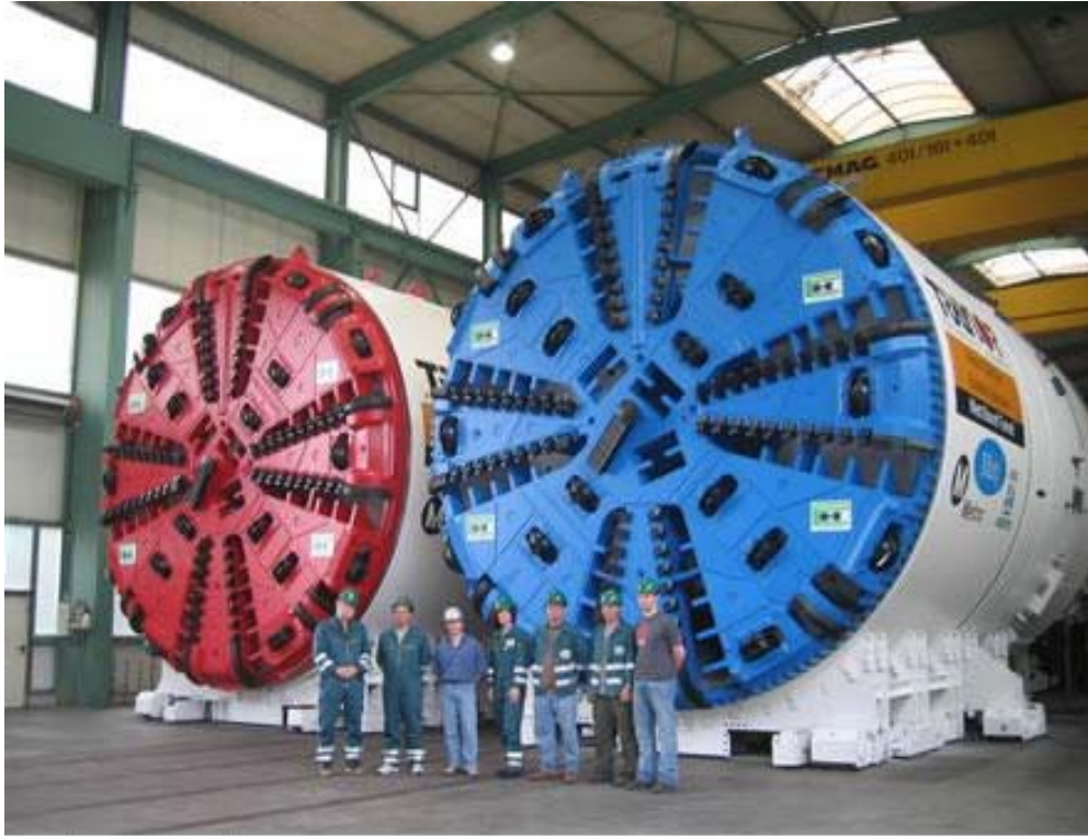
Gold Line Eastside Extension Project - utilizing two German-manufactured tunnel boring machines
